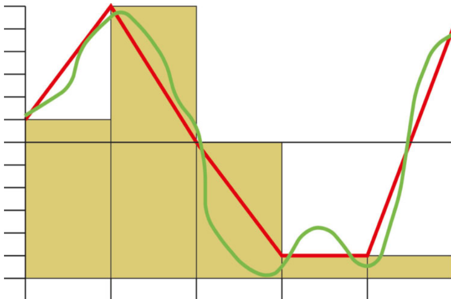
▲ Figure 2: Sampling the waveform with a slow sample rate and high accuracy.
