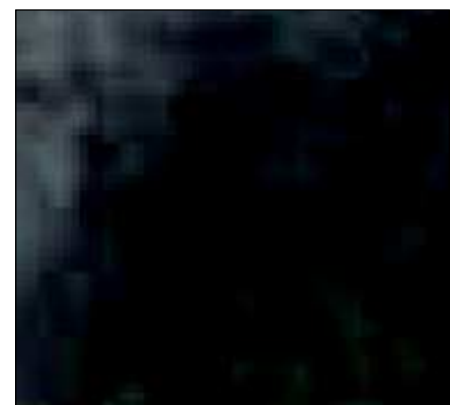
▲ Figure 3: Typical JPEG block artifacts caused by the compression algorithm (magnification x7).
